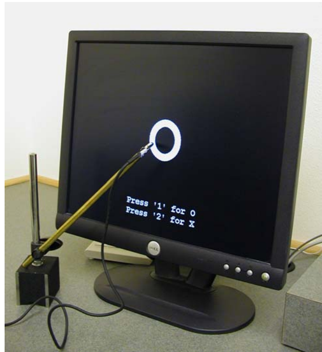
Figure 2-9. The photocell holder positioned for a visual-stimulus experiment
