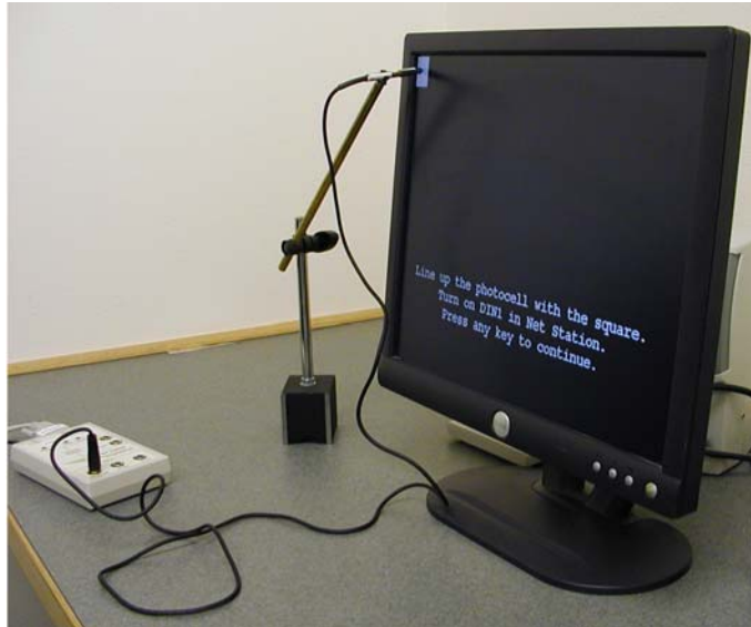
Figure 2-7. The photocell holder positioned for the NSTimingTest.es file
